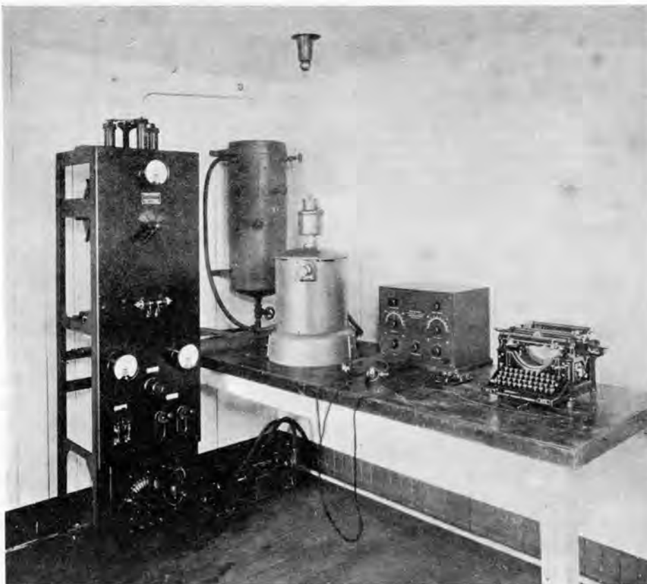
Typical ship installation of a Federal Telegraph Company 2-kilowatt arc transmitter.
